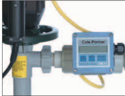
Batch control pump systems include a programmable controller; set and display dispense volumes and monitor total volume dispensed.
